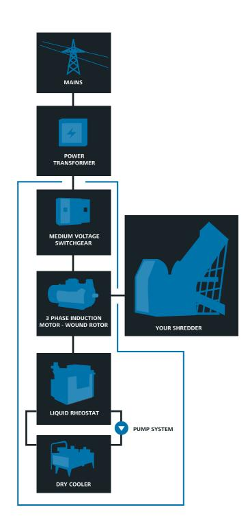
We deliver your complete drive system from liquid rheostat and switchgear to wound rotor motor and dry cooler for your shredder, in accordance with your demands.
