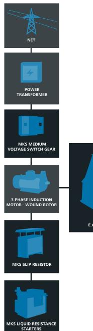
We deliver the components for your drive system – liquid resistance starters, switch gears and slip resistors customised according to your needs.
